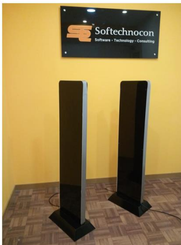
Wireless UHF RFID Scanner with Scanning Range of 3 to 4 Feet from single Pillar
